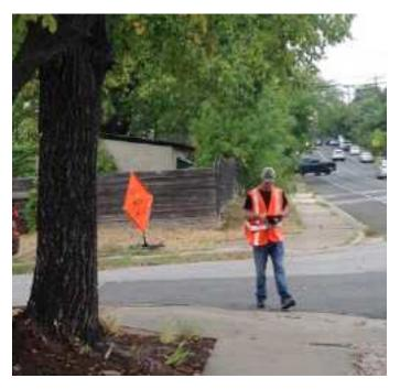
A field team using GPS handheld devices to efficiently pinpoint and delineate critical environmental features as part of a municipal tree survey. Data collected was used to create a GIS-based field inventory of tree species by type, size, age and relative health.
